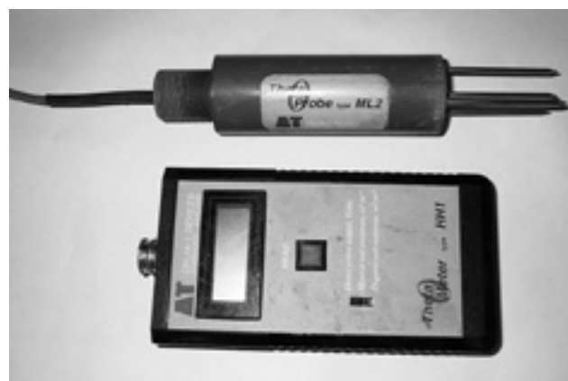
Figure 3. Theta probe by Delta-T technologies.
