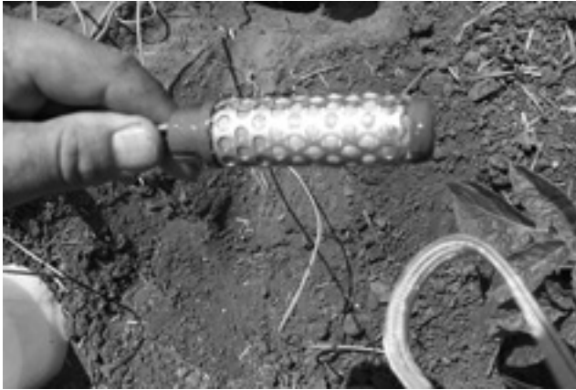
Figure 4. Watermark sensor by Irrometer.
